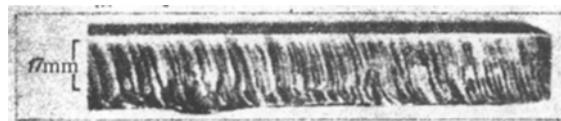
Fig. 3. Photograph of the lateral surface of the metal strip after plasma cutting.
